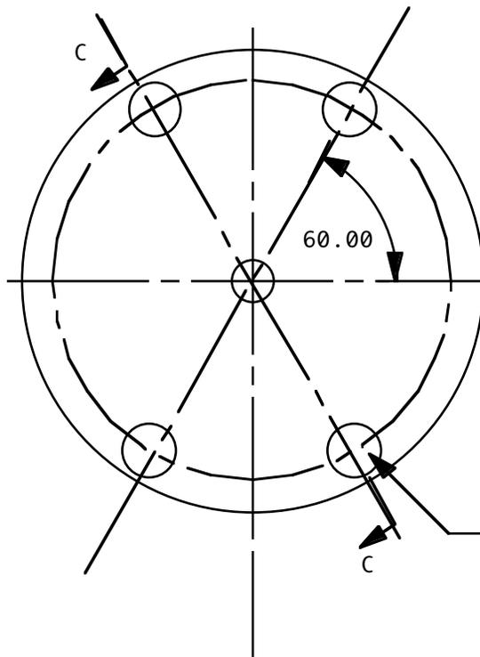
Drill thru, 4 holes 5/16" placed as shown on a 2.375" dia circle as shown to within 0.001" of true position. Part D will key into holes
